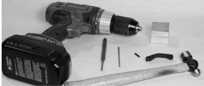
[1] Remove the current trigger guard using the 1/8" punch; depress the front detent spring and rotate the trigger guard down, clear of the receiver. Using the same punch, drive out the rear roll pin for use in the re-installation of the replacement trigger guard.
