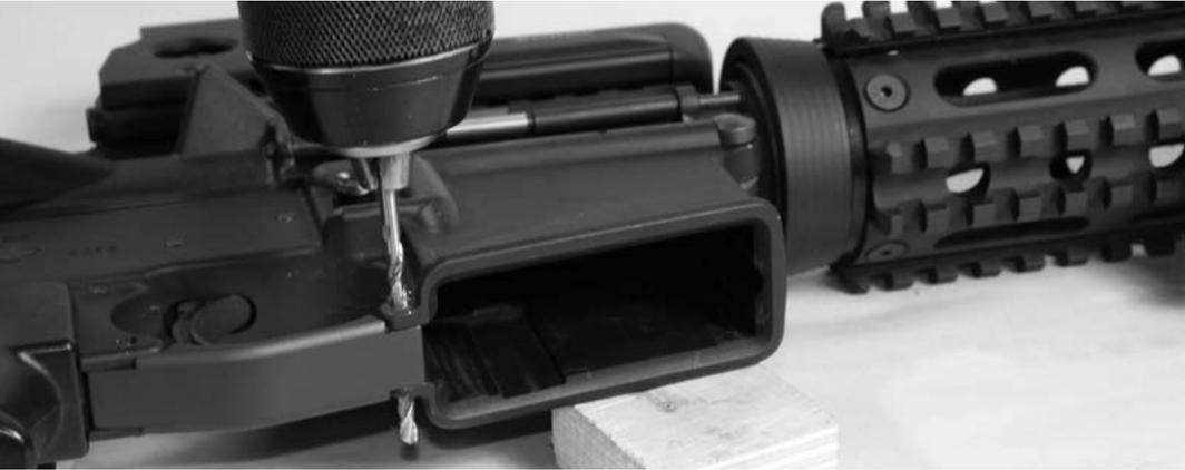
[3] Align the front hole of the trigger guard with the existing hole in the receiver. Using the No. 30 drill bit, drill through the entire trigger guard hole until the drill bit passes through the bottom side of the receiver. Make sure the trigger guard holes align. This will ensure a straight hole from top to bottom.
